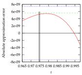
$\begin{array}{c} \text{Approximation error} & ----\\ \text{Required bound } 2^{-25}/(4-2^{-21})\approx 8\cdot 10^{-9} & ----\\ \text{Approximation error bound } \theta=3\cdot 2^{-29}\approx 6\cdot 10^{-9} & ---- \end{array}$
