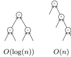
**Figure 1: Graphical representation of Algorithm 1 and Algorithm 2 by dataflow graphs.**
