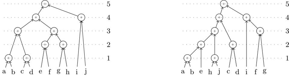
a) Fully Parallel and Non-Fully Accurate Algorithm. b) Fully Accurate and Non-Fully Parallel Algorithm.
